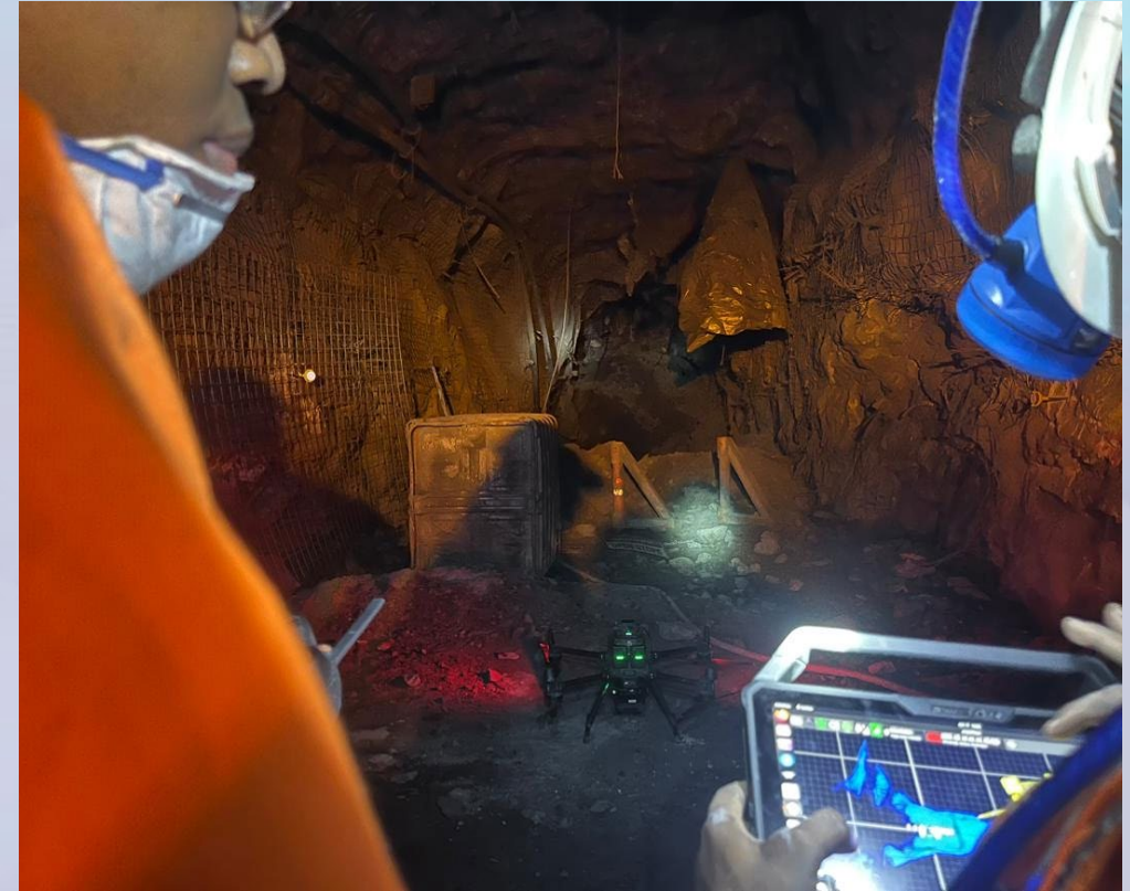
Figure 18 Drone Setup at a safe distance from the stope
