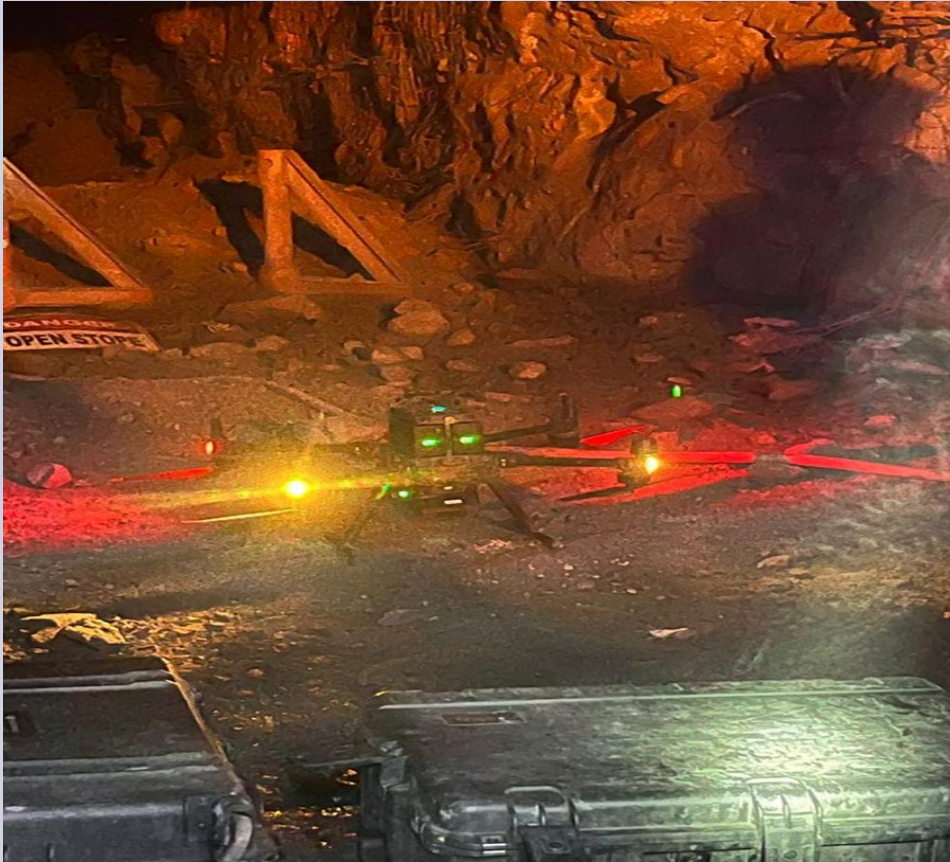
Figure 2 Underground Drone equipped with a LiDAR-SLAM scanner
