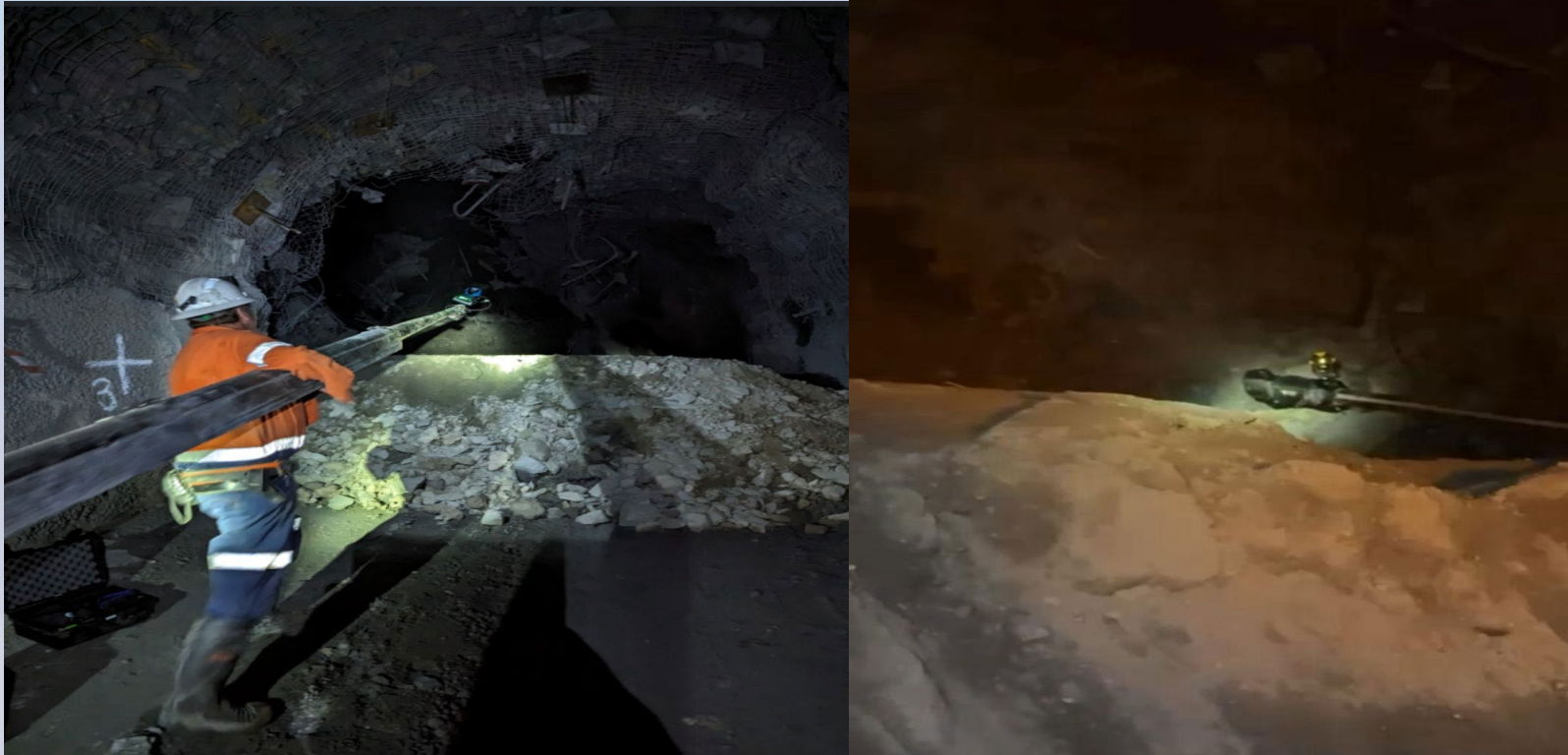
Figure 17 CMS Setup at the brow of the stope
